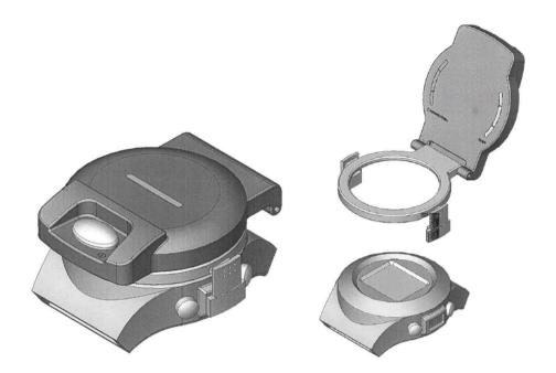
This prototype was made as a proof of concept for the BPro G2.<sup>243</sup> Although this prototype BPro G2 was functional using the wireless Bluetooth technology, it was bulky and the design had to be greatly enhanced to make it aesthetically acceptable for the market.
