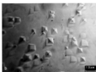
Figure 6: Etch pits on diamond with dislocation density of 3300/\text{mm}^2
