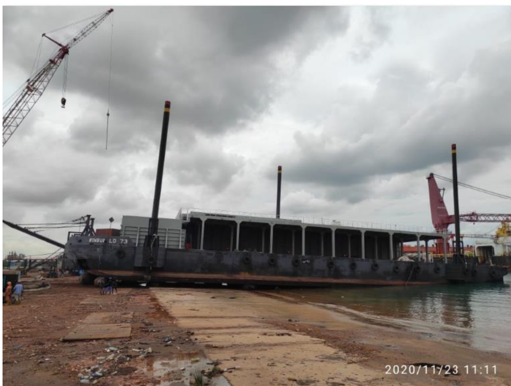
Figure 3A: Photo of the "WINBUILD 73" with three spud legs
